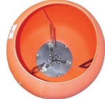
6 cu. ft. drum. Rotates 28 times per minute. Mixes 5-60 lb bags of premixed concrete
