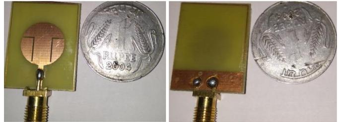
(a) Front and Back view of Proposed Antenna Prototype
