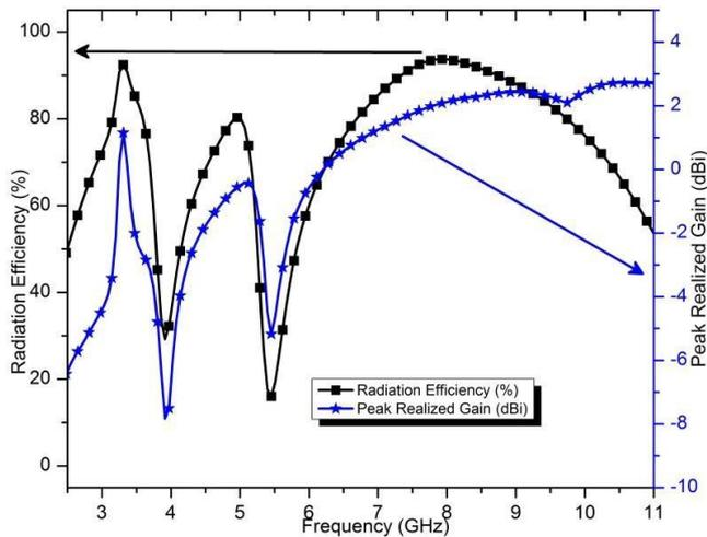
Fig.11. Radiation Efficiency and Realized Gain of Proposed Antenna
