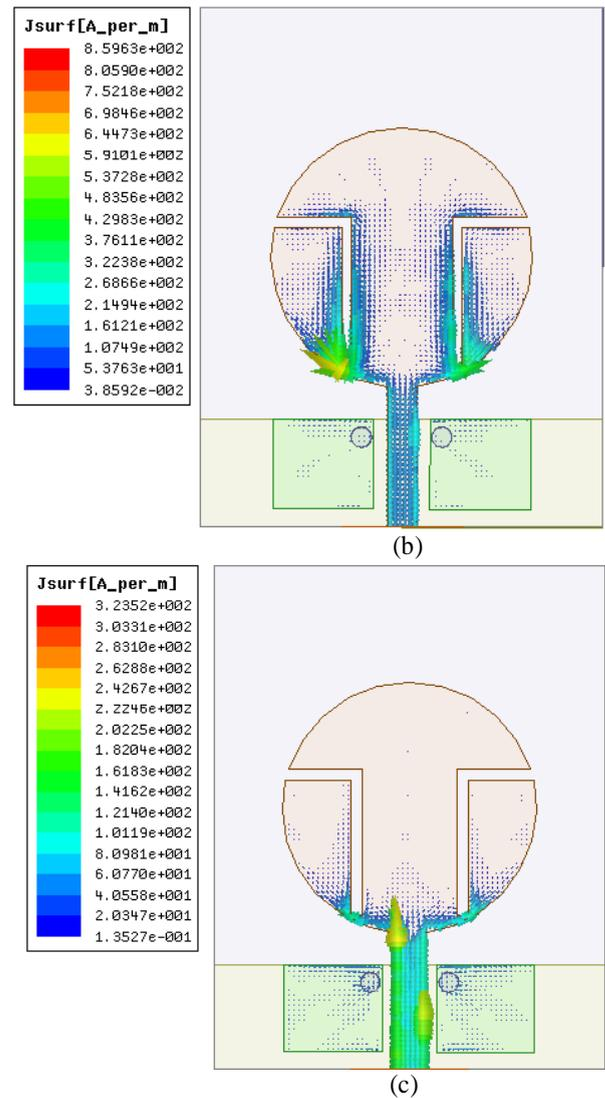
Fig.8. Current Distribution (a) 5.5 GHz, (b) 4 GHz and (c) 7.5 GHz
