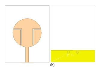
Fig.1. (a) Front View and (b) Back View of Proposed Antenna
