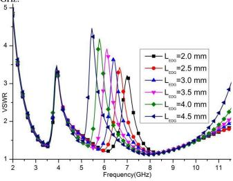
Fig.4. VSWR variation due to EBG Length. Width optimization of the proposed EBG has been present in Fig.5. From Fig.5 it can be seen that the EBG width has a great impact on the frequency tuning of the proposed antenna. The width of the proposed EBG is function of frequency. It can be verified from the Fig.5 that center frequency of band notch inversely varied with the EBG width.
