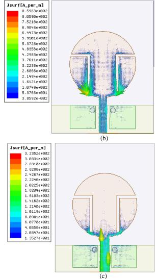
Fig.8. Current Distribution (a) 5.5 GHz, (b) 4 GHz and (c) 7.5 GHz
