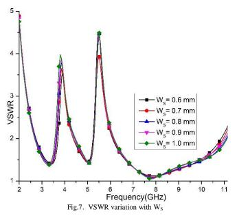
From above optimization processes of SRASP slot, we can say that to create tunable band notched, EBG structure approach is better over conventional slot methods.
