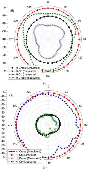
Fig.10. Measured and Simulated, Normalized E & H field patterns of proposed antenna (a)E-field at 4.5 GHz (b) H-field at 4.5 GHz (c)E-field at 6.5 GHz (d) H-field at 6.5 GHz
