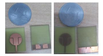
(b) Front view, Sandwiched EBG and Back view Fig.2. Fabricated Prototype of Proposed Antenna
