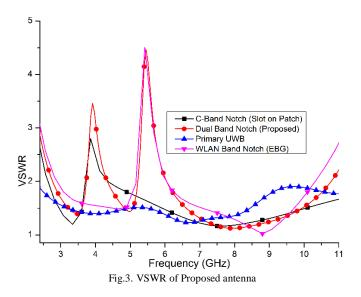
The length and width of the mushroom shape EBG played a crucial role in optimization of proposed antenna. We have varied the length and width of the EBG structure over a range. The optimization of  $L_{EBG}$  and its effects on VSWR result have been shown in Fig.4. From Fig.4, it can be observed that band notch frequency is a function of length of the EBG structure and it varies inversely with the length. However, we have tuned the length of EBG for WLAN band center frequency 5.5 GHz.
