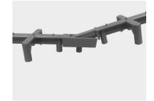
**Art Mould's Slab Bolsters** provide high weight load support for slab, precast, post-tension, tilt-wall and parking garage applications. Available in 30" lengths, they are lightweight, can be used individually, or snapped together with a unique clip designed for easier and quicker installation. Leg spacing is 2 1/2" with 1" bar guides and the arch design maximizes strength to reduce deflection between legs.
