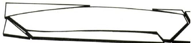
ways: (1) If your design fits closely to the outside proportions of your blade steel, you may choose to grind away all the excess steel down to the scribe lines of your design; (2) You can drill a hole around and to the outside of your scribe lines. Then take a hacksaw and cut your design out; (3) Take your blade steel to a machine shop and for a nominal fee have them cut out the design on a metal cutting band saw. Always remember to cut just to the outside of the scribe line.
