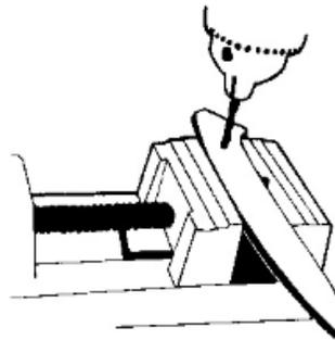
Since we will be using a screw-type rivet (actually a bolt-on rivet) we will have to use a 3/16" drill bit. Chuck this in your hand-drill or drill press, and drill the rivet holes. When you use a hand-drill, place the blade steel upright in a bench vise
