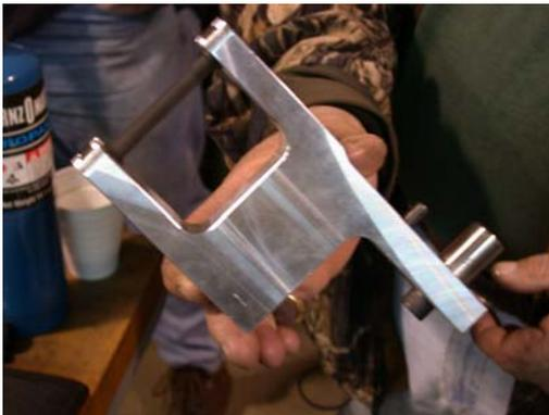
This grinder attachment is used for grinding the small radius.
