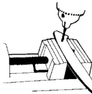
Since we will be using a screw-type rivet (actually a bolt-on rivet) we will have to use a 3/16" drill bit. Chuck this in your hand-drill or drill press, and drill the rivet holes. When you use a hand-drill, place the blade steel upright in a bench vise for easier handling. If you use a drill press, either clamp the steel to the drill press table or clamp it in a drill press vise. Always remember to wear protective glasses when using any power tools.
