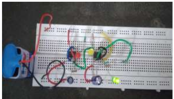
Fig. 5. Experimental setup of traffic light controller with green color glowing
