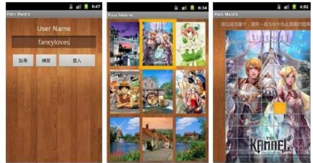
Fig. 11. (a) The Main page of PassMatrix, users can register an account, practice or start to log in for experiment. (b) Users can choose from a list of 24 images as their pass-images. (c) There are 7 × 11 squares in each image, from which users choose one as the pass-square.
