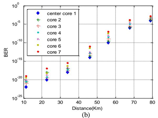
Fig.2: Simulation results of BER performance w.r.t distance of 11.3km using TA-UMCF at 7 spans (a) BER performance w.r.t distance for downstream (b) BER performance w.r.t distance for upstream
