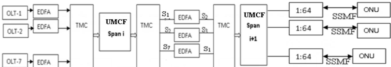
Fig.2: Block diagram of passive optical network system with hybrid fiber (TA-UMCF and SSMF)
