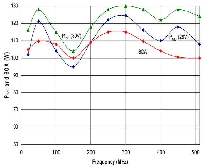
**Figure 4: RFM20-512-100 Typical  $P_{1dB}$  @ 28VDC and 30VDC, and Safe Operating Area (SOA). Do not exceed the SOA shown above without first contacting RFMPT to discuss your application.**
