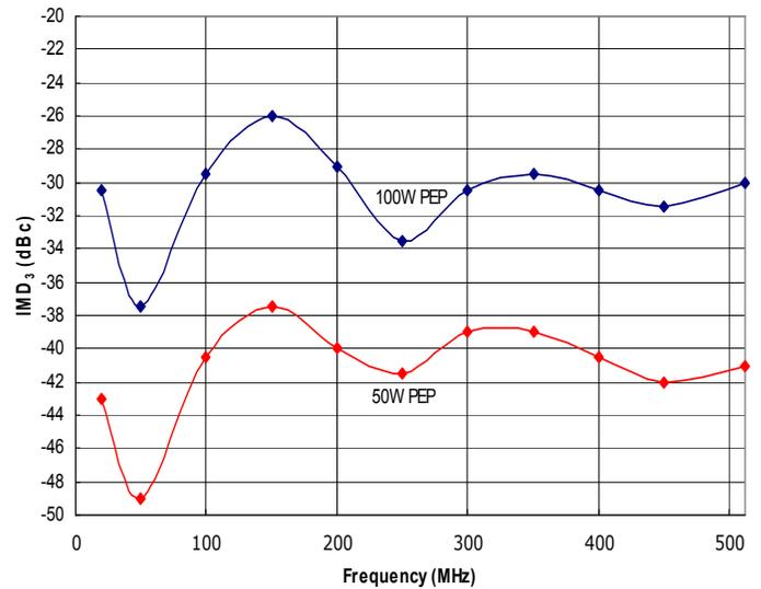
**Figure 2: RFM20-512-100 Typical  $IMD_3$  @ 100W and 50W PEP,  $\Delta f=10kHz$ .**
