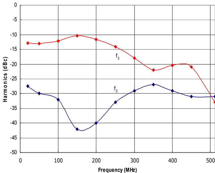
**Figure 3: RFM20-512-100 Typical  $f_2$  and  $f_3$  @  $P_{out}=100W$ .**
