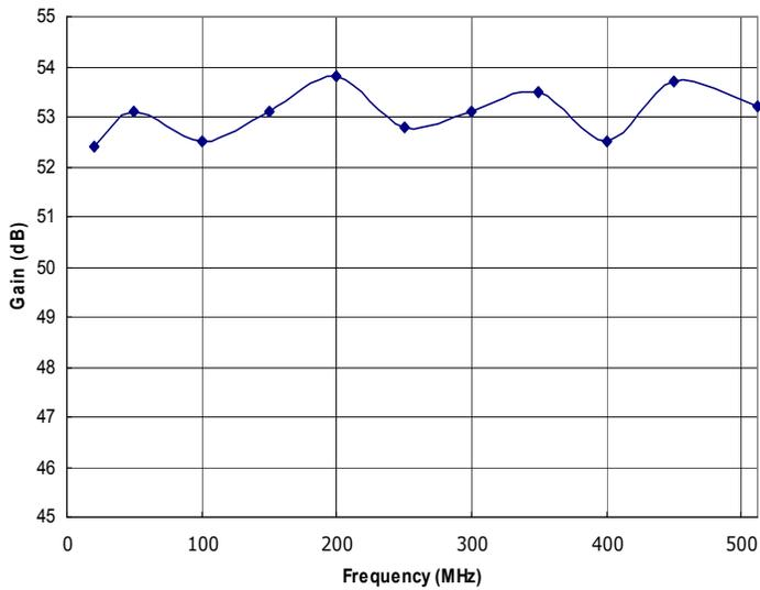
**Figure 1: RFM20-512-100 Typical Gain @  $P_{out}=100W$ .**
