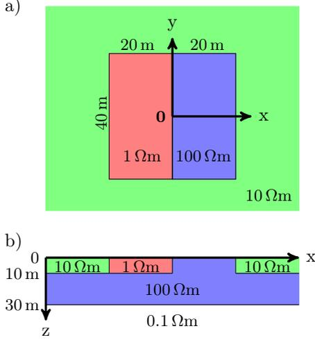
**Figure 1:** Plan view (a) and slice (b) of the 3D-2 COMMEMI model.
