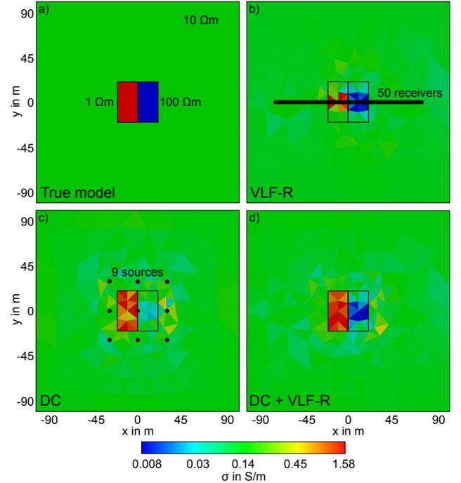
**Figure 2:** Plan view of the downscaled 3D-2 COMMEMI model. a) The true model used to compute the synthetic data. b) and c) are the inversion results for the individual VLF-R and DC resistivity inversion, respectively. d) Using the DC resistivity solution as the reference model, we then inverted the VLF-R data to obtain a joint inversion result, which recovers the two anomalous bodies well.
