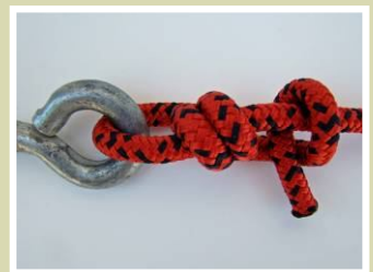
Make a half hitch on the opposite of the first two in the same direction
