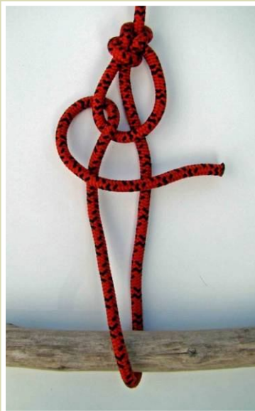
Make a turn on an anchor point bringing the working end through the bowline loop.
