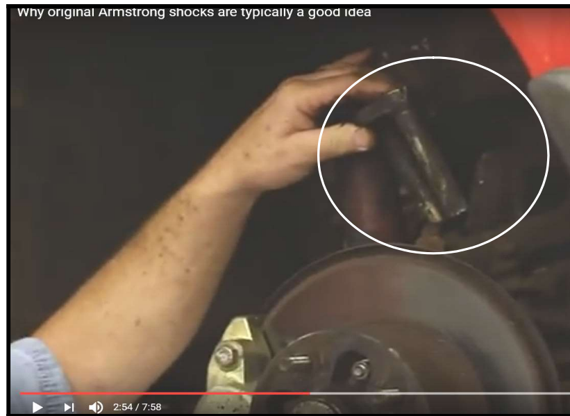
Figure 36 - Damaged Support Bracket
