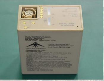
discharge 20.0A in 12V mode, 10.0A in 24V mode Max pulse discharge 36.0A in 12V mode, 18.0A in 24V mode Nominal dimensions 62 x 112 x 127 mm Nominal weight 1.30kg Connector Floating type per U.S Army DWG # SC-C-179495 Case material Modified ABS, desert tan Operating temperature -20oC to +60oC Shelf Life Five (5)
