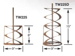
**TW225** – for half batches (2-3 bags); 9" diameter x 27" long; ideal for plasters, concrete, mortars, resins and tile adhesives. 8" long helix and side bars.
