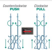
**Counterclockwise** rotation pushes material from the top to the bottom, reducing splashing when mixing low-viscosity materials such as paint, glue, filler and leveling compounds.
