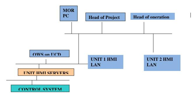
Figure 1: Typical DCS/PLC network in a power plant
