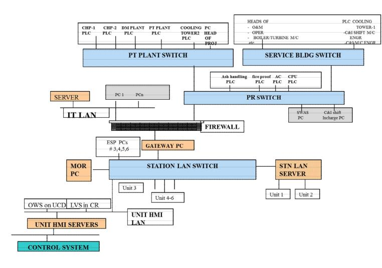
Figure 2: Typical DCS/PLC network in a power plant
