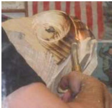
Next step is coloring done with the use of a blow torch. Our owl was turned from ash which with it's coarse grain allowed detail to be enhanced with burning.
