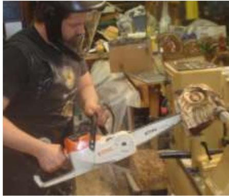
Derek has a battery operated Stihl chain saw with which he removes material from the inside of the head. Derek likes to keep about an inch and three quarters for the inside wall thickness. He says it helps prevent warping and distorting this way as the wet wood dries. Also with wet wood, it allows for more controlled burning whereby only the top or high points of the wood surface are burned rather than torching the entire surface.
