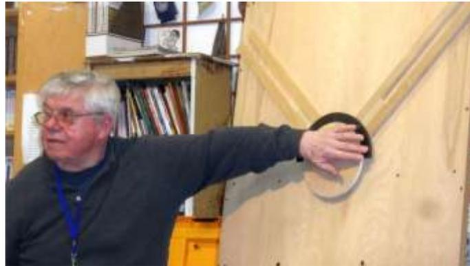
Bob used a board with simulated chuck jaws to show us what can happen if a piece is too large to be supported by the chuck on the lathe.
