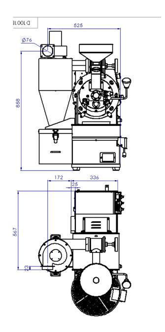
THE ORO 4 COMES STANDARD WITH THE M4 SYSTEM WITH 4 DEDICATED MOTORS AND TWO EXHAUSTS. THE TOP PIPE OFF CHAFF UNIT IS 3" & THE PIPE SIZE FROM COOLING TRAY IS 5".
