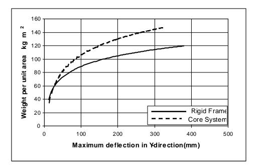
Figure (10): Relationship between steel weight and deflection in Y-direction
