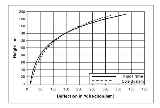
Figure (7): Relationship between height and deflection in Y-direction
