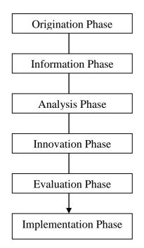
Figure (1): Phases of Value Engineering Process
