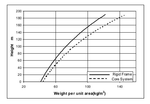
Figure (8): Relationship between height and material weight per unit area
