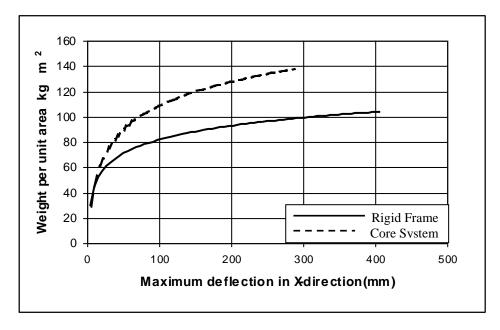
Figure (9): Relationship between material used and deflection in X-direction
