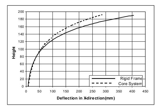
Figure (6): Relationship between height and deflection in X-direction
