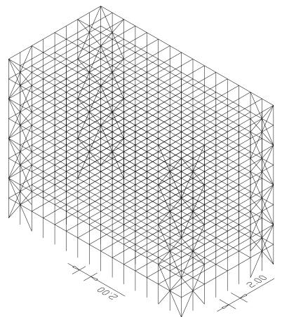
Figure (4): Lateral load resistance using tube system
