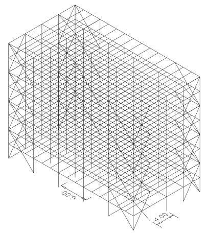
Figure (3): Lateral load resistance using rigid framing system
