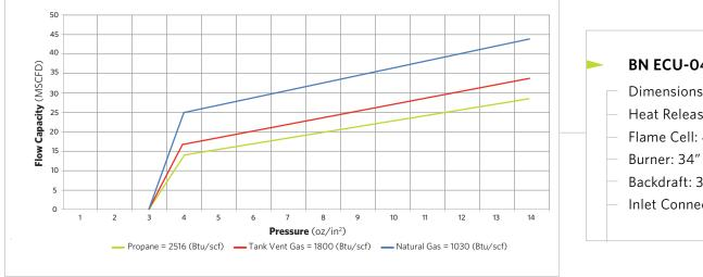
**BN ECU-048** Dimensions: 48"D x 8'L Heat Release: 2 MMBTU/hr. Flame Cell: 48"
