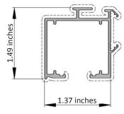
Coating perimeter: 7.5 in (see Dashed Line) Anodised perimeter: 313 (Total Perimeter)
