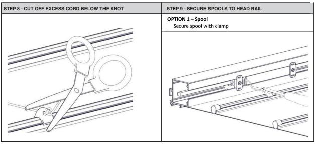
$^{\star}$  Quick tip: Leave 3" of cord to allow further adjustments to be made by installer
