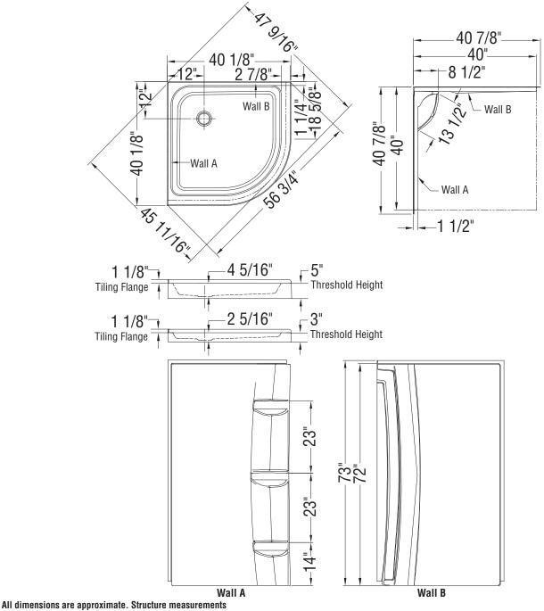
must be verified against the unit to ensure proper fit.
