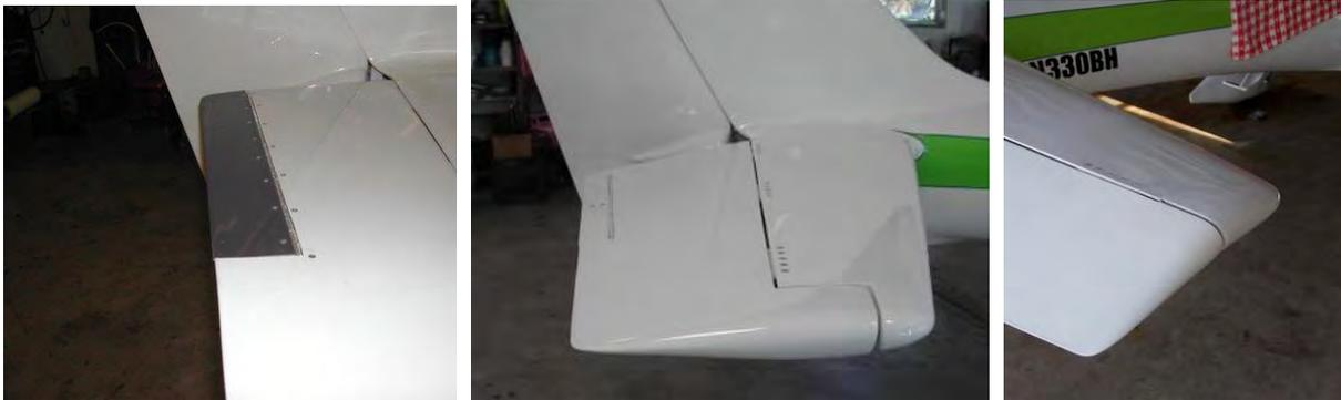
**In the photos above, you can see the larger trim tab and the aerodynamic elevator counter balance that Bob mentioned. On the left photo is the new larger trim tab. The center photo shows the original trim tab and the elevator aero counter balance. The right photo is the latest configuration without the aerodynamic counter balance. It was found that the counter balance made the Lightning a little too sensitive for most people's flying experience.**
