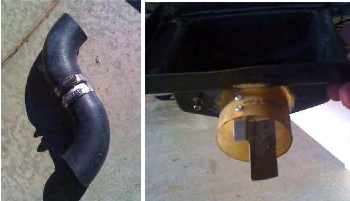
**Dave's photos above, showing the smooth rubber tube that replaced the scat hose and the aluminum plate he installed in the air box outlet are easy to understand. However, I am still not sure how the spacer, that appears to be around the air filter, actually moves the air filter 1/2" out from the firewall. A message to him asking for more info resulted in the message below.**
