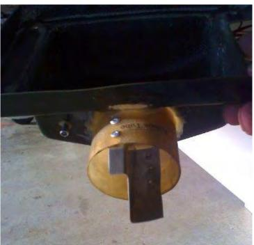
Dave's photos above, showing the smooth rubber tube that replaced the scat hose and the aluminum plate he installed in the air box outlet are easy to understand. However, I am still not sure how the spacer, that appears to be around the air filter, actually moves the air filter  $\frac{1}{2}$ " out from the firewall. A message to him asking for more info resulted in the message below.
