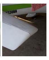
In the photos above, you can see the larger trim tab and the aerodynamic elevator counter balance that Bob mentioned. On the left photo is the new larger trim tab. The center photo shows the original trim tab and the elevator aero counter balance. The right photo is the latest configuration without the aerodynamic counter balance. It was found that the counter balance made the Lightning a little too sensitive for most people's flying experience.
