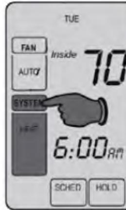
2. Press, and Hold the 3rd and 5th Buttons Simultaneously
