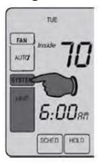
2. Press, and Hold the 3rd and 5th Buttons Simultaneously
