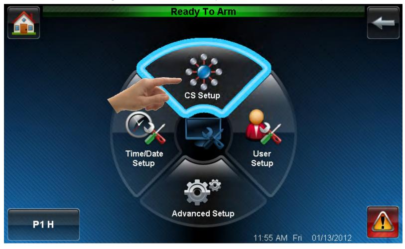
• Enter the Panel Installer Code. The TUX Internal Installer Code is 4140.
