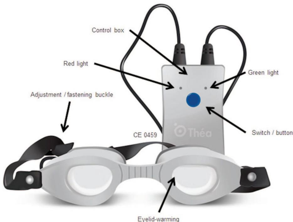
**FIGURE 1.** The Blephasteam eyelid-warming device. Reproduced with permission from Laboratories Thea. A color version of this figure is available online at [www.optvissci.com](http://www.optvissci.com).
