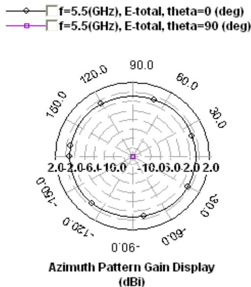
Fig. 5. Radiation pattern for azimuth plane
