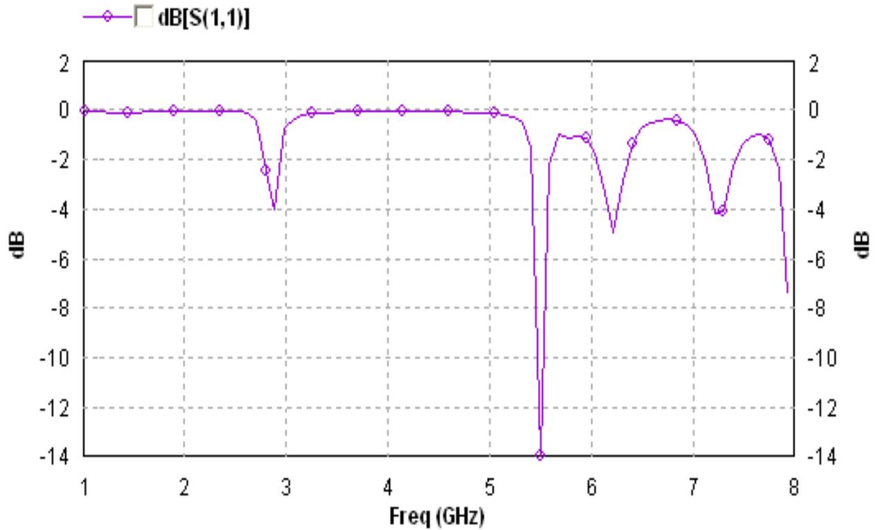
Fig. 2. Return loss of proposed antenna
