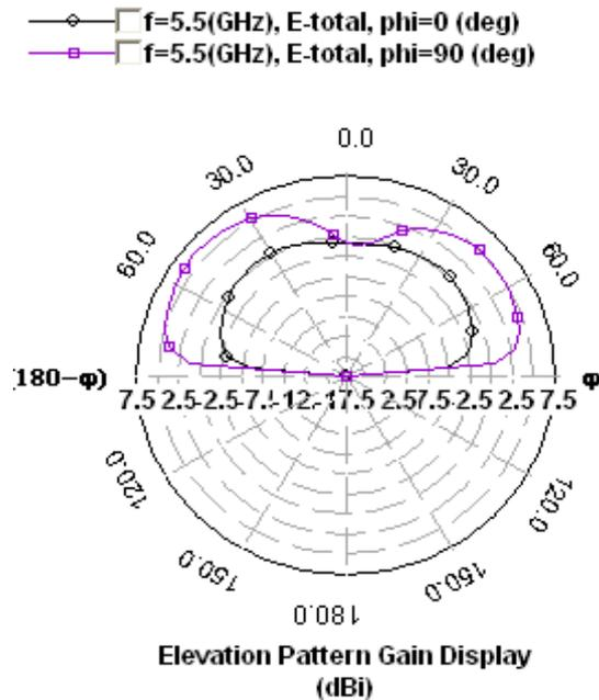
Fig. 4. Radiation pattern of elevation plane
