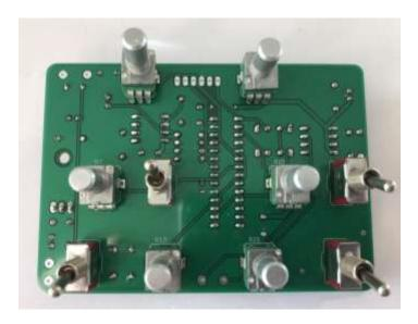
22. With the switches and potentiometers on the PCB, gently push them into the aluminum box.
