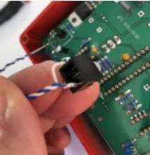
26. In the pictures above, the white wire is the audio ground wire and the blue wire is the audio output. As per the picture below, solder the audio out wire to the pad marked A.OUT and the audio ground wire to the pad marked A.GND.
