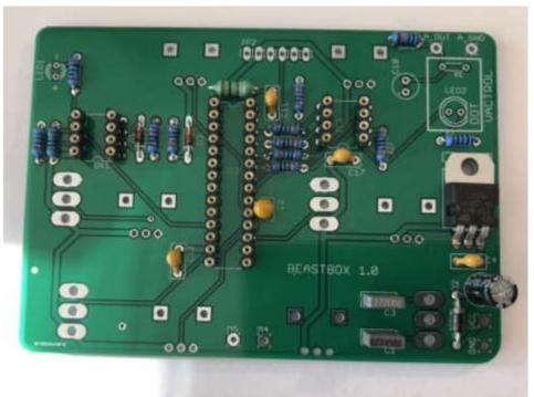
17. Install the 10uf electrolytic capacitor C18 – these capacitors are polarized and must be installed with the longer lead into the hole marked with the + symbol.
