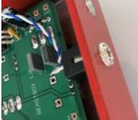
27. Now its time to connect the power socket. Cut and strip a piece of red wire and a piece of black wire. Solder them onto the socket as per the pictures below – the third lug on the socket is not used and should be cut off with a pair of side cutters.
