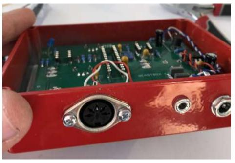
31. Once the wires are complete its time to install the IC's (IC2, IC3 and OK1). IC's must be installed in the correct direction. There is either a dot or a notch on the IC to indicate pin 1. There is also a notch on the PCB silkscreen to indicate pin 1. Make sure the notch/dot on the IC package matches the silkscreen on the PCB.
