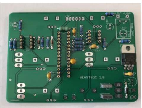
16. Install the 100uf electrolytic capacitor C20 – these capacitors are polarized and must be installed with the longer lead into the hole marked with the + symbol.
