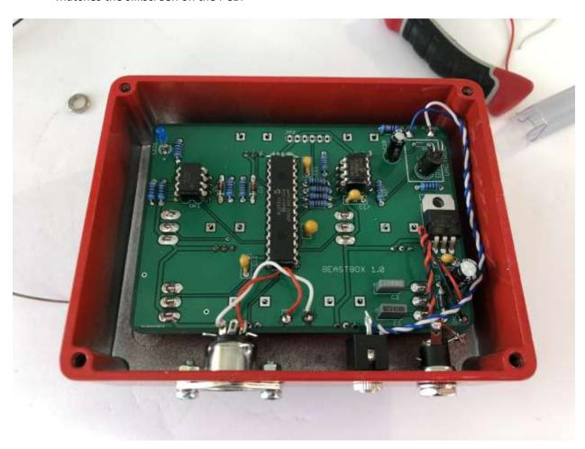
32. Flip the box over and install the knobs. Turn the potentiomenters fully counter clock wise, then loosen the grub screw on the knob, place on the potentiometer and tighten as per the photos below.
