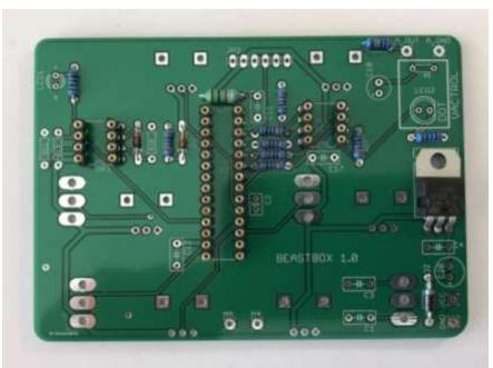
9. Install the 220 ohm resistor R10 ( red red black black brown ) and solder into place.
