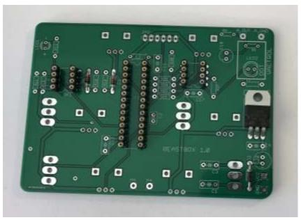
5. Install the seven 10K resistors (R18, R23, R24, R25, R26, R27 and R30) and solder into place.
