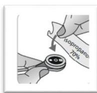
Verify that the sensor is clean before changing its membrane. If necessary, carefully wipe off any residue from the sensor’s surface (including membrane, housing, groove, and cable) with 70% isopropanol.
