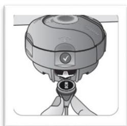
Press one last time or lift the sensor and remove it from the Membrane Changer. The ✓ symbol indicates that the membrane change is completed.
