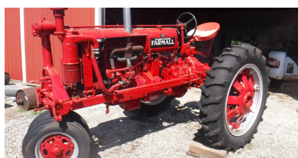
Lot 1 1939 Farmall F20 Tractor has been overhauled. Paints & New Tires. New Modine Radiator Core and aftermarket K&M 5th Gear.
