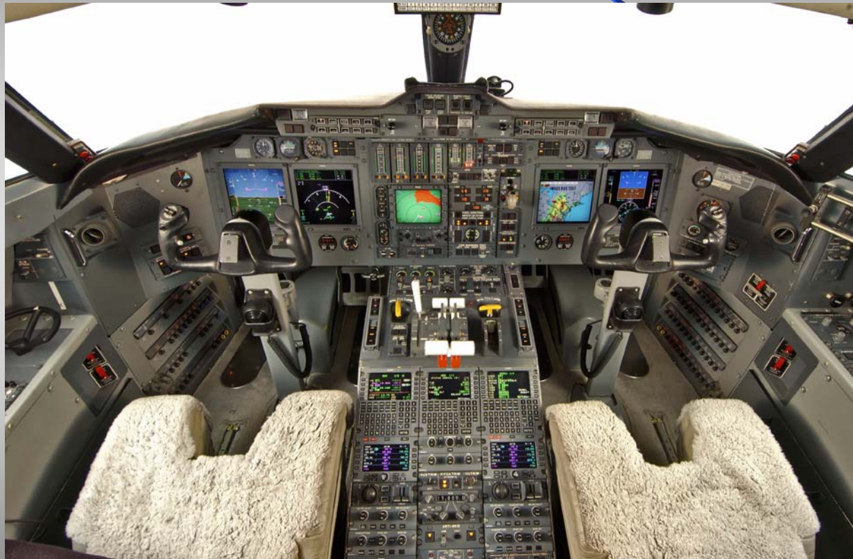
Flat Panel Retrofit UASC R890 completed in Sept. 2004
