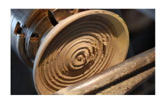
Finish hollowing then sand and finish the inside of the bowl and the first ¼ inch of the outside rim.
