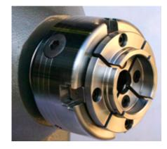
There are several design jaws, dovetail, toothed, and multi toothed. I prefer the Nova chuck jaws that are dovetail on the outside and have one tooth on
