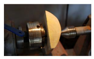
made the blank approximately as long as it is wide. I placed the cut flat center of the log against the chuck jaws and held in place with the tailstock and rotated and adjusted to center.
