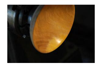
Put a small Formica covered faceplate in the chuck and place the open side of the bowl against the faceplate, use the live center to center the bowl on the faceplate. I left the center mark made earlier which allows me to center the work exactly.
