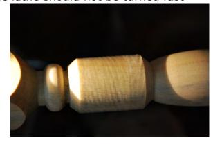
the surface of the wood, that is because there are differences in hardness of the wood (late wood, early wood) and the speed of the wood past the tool allows the tool to "dip" into the softer wood then "bounce" out when the harder wood comes by this leaves a low spot and a high spot. When these come around again it amplifies the dip and bump and creates a new one a little later in the rotation and on and on and on... What do you about these,
