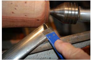
restore the edge many times before you need to regrind the skew. When the little flat spot, or mini bevel, is 1/16" to 1/8" you should consider regrinding.
