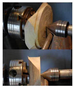
I will continue the line of cut till the blank is round and has straight sides.
