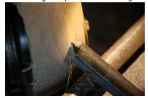
cut and the finish cut is both the angle of the tool and the pressure on the tool. A **finishing cut** will have much less pressure on the tool and thus on the wood and the angle of the cutting edge where it meets the wood may be
