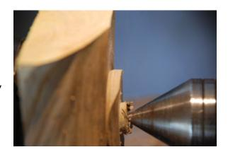
I then mounted the blank in the jaws by the spigot with pressure from the tailstock to help set the jaws while tightening and providing a little extra safety while knocking off the corners.
