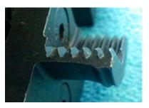
easier to make the spigot that fits these jaws. When you make the spigot to grip on the outside remember to make room for the tooth, if you don't it will try to bite the spigot off of the bottom of the bowl, and it will be successful more often than you would like it to be. The spigot should never touch the inside bottom of the jaws, always make the spigot so that the wood registers against the outside top of the jaws.
