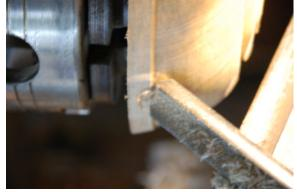
cracks extend into the wood from 1/16" to over ¼", and that is why you can't sand them out! I like to practice the finishing cut while roughing out the center of the bowl; it is a delicate balance between "hogging" out the wood and cutting out the wood. Practice, you will find that spot between making a rough cut and a smooth cut.
