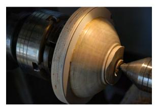
Then a little dab of hot glue to hold the bowl to the faceplate and you can finish the outside of the bowl and the foot. The foot is made by making a cove in the center of the foot.
