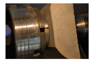
Here you see the blank starting to get to round. Notice that I am turning starting at a smaller diameter and turning to a larger diameter, a supported cut, to get a smooth cut.
