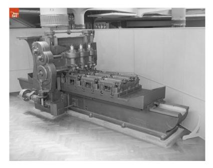
At 21 feet long and 8 feet tall, this was no small milling machine. There are two inscriptions on the machine:
