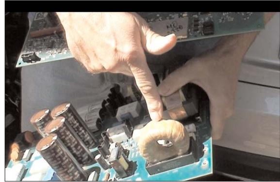
Ron points to an induction coil that gets hotter than 250 °F. He can frequently troubleshoot these boards by using a heat sensor that can indicate whether or not the component is working. No heat (a cold heat sink) can indicate that an item like a transistor is not working.
