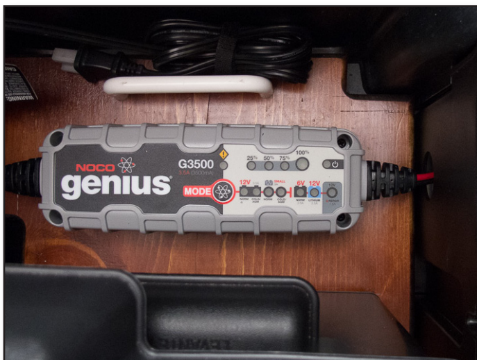
FIGURE 4: The battery charger in position and the charging cord routed through a hole in the slots in the back of the box.
