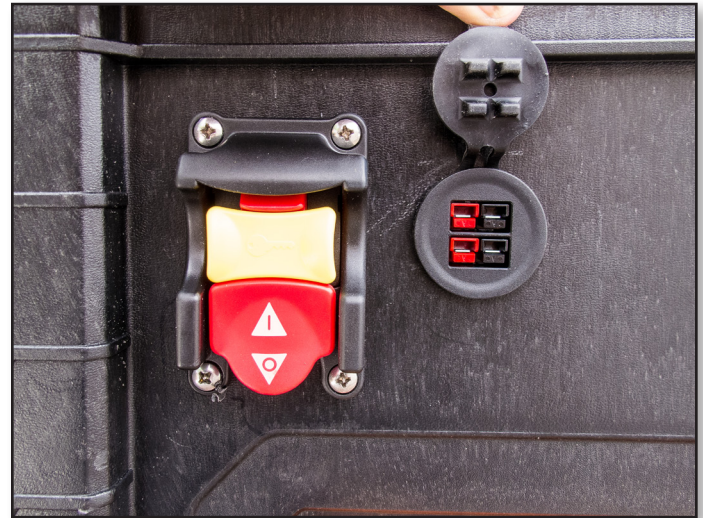
FIGURE 6: The main power switch and the Powerpole® socket installed on the front of the box.
