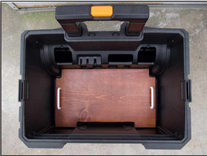
FIGURE 2: The component mounting board cut to fit and located in the bottom of the tool box.
