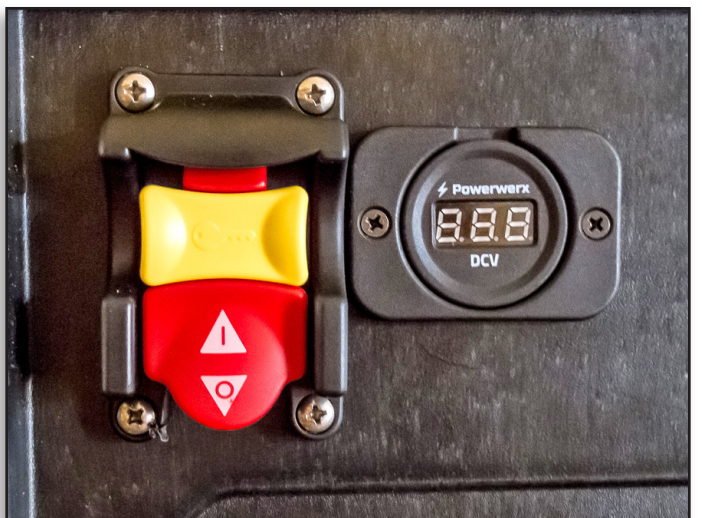
Figure 12: Main power switch and voltmeter that replaced the Powerpole socket on the front of the box.
