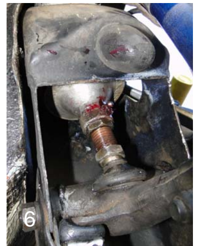
Photos 5 & 6- All finished with the coil spring conversation, just needed to put the wheels back on and check the ride height.
