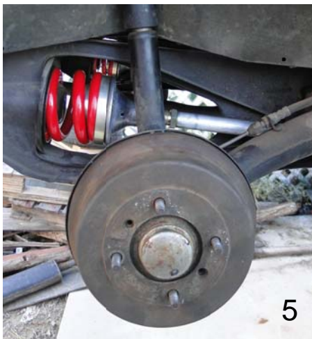
Photos 5 & 6- All finished with the coil spring conversation, just needed to put the wheels back on and check the ride height.
