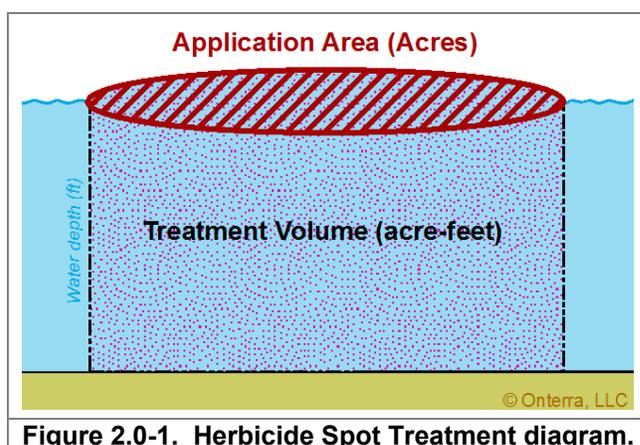
Figure 2.0-1. Herbicide Spot Treatment diagram.
