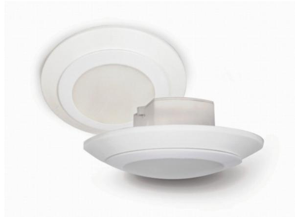
Another option are LED light discs. Light disc are thin circular discs with LED lamps inside. Light discs can be purchased as a retro fit style, installed inside an existing pot light. These are purchased based on the size of the pot light and fit inside using springs and clips to secure them. Light intensity is also higher as the size goes up.
