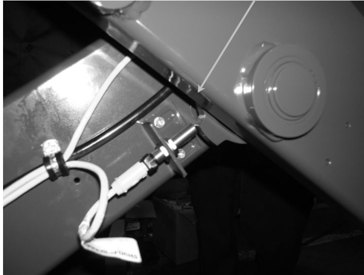
Figure 16 - Upper limit proximity sensor
