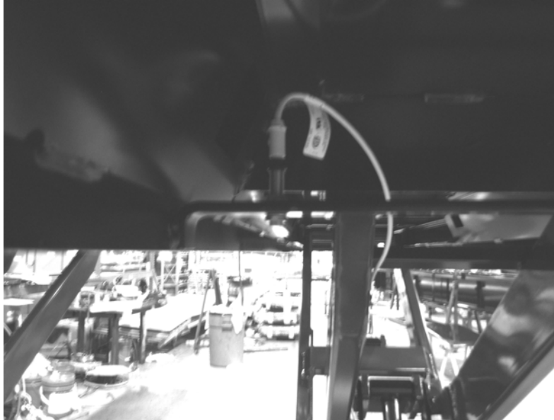
Figure 17 - Equalizing proximity sensor Under front of deck
