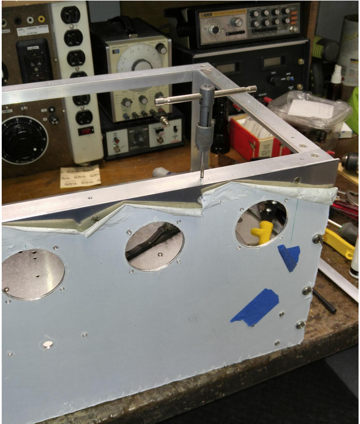
Figure 13: Tapping Holes in Cabinet Frame
