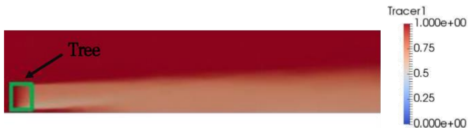
Fig 4 - A passive tracer is advected from the left of the domain. A porous tree is located in the domain. The pollution is absorbed and reduction of concentration can be observed downstream the tree.
