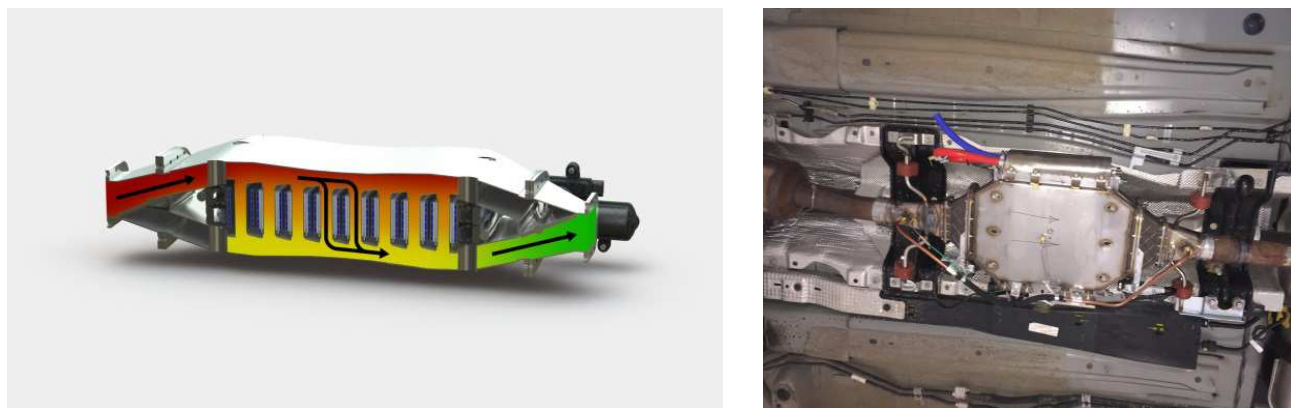
Figure 9 (a) Image of VIPER2 thermoelectric module for vehicle application, (b) VIPER2 module fitted to underside of test vehicle. Both images courtesy of the Innovate UK funded VIPER2 programme.
