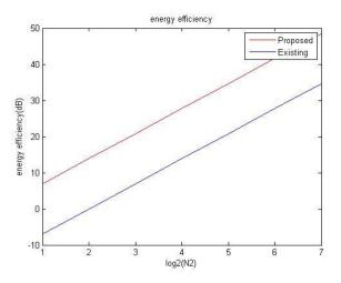
Fig 5.7 Energy efficiency Vs order of the hadamard transform
