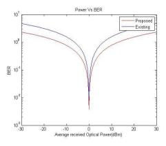
Fig 5.5 Power Vs BER for M= 512
