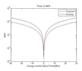
Fig 5.2 Power Vs BER for M= 8
