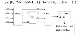
Fig.1 Block diagram of HCM transmitter
