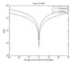
Fig 5.4 Power Vs BER for M=32
