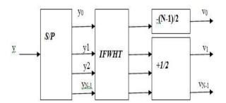
Fig.2 Block diagram of HCM receiver
