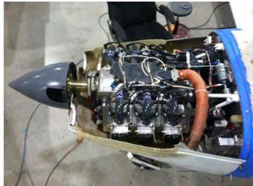
**Left- Doug and Ronda's ULpower 390 160hp Lightning just back from the paint shop. Right- UL390 install almost finished.**
