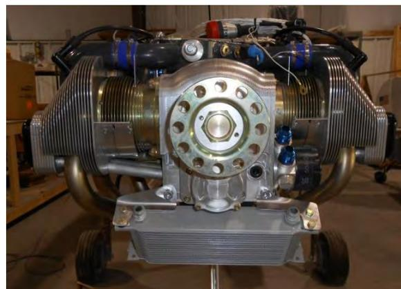
**The above four photos show the ignition coils and high pressure pumps mounted on the firewall and the oil cooler mounted on the front of the engine.**
