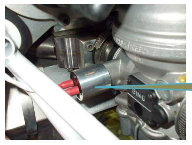
The heating element should be wired to the electrical system of the aircraft via the main bus bar and protect by a 10 amp fuse and switch.
