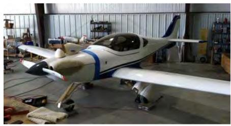
N958DG up on the scales. UL390is 160hp. 925lbs empty all up, has GRT 10.5" HXR system with AP, GRT back up battery, VP-X pro, dual Aerovoltz 16cell lithium batteries.
