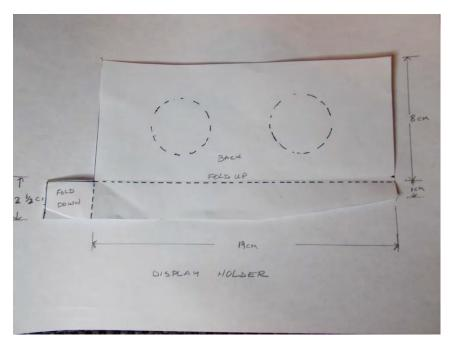
The two circles represent the speaker locations on the IFLY and can be cut out or, as an option, you can easily cut the display at the mid-section of the circles straight across. It would still be capable of holding the IFLY and giving you some speaker sound. (you probably won't hear much in the cockpit anyway...)
