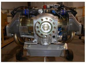
The above four photos show the ignition coils and high pressure pumps mounted on the firewall and the oil cooler mounted on the front of the engine.
