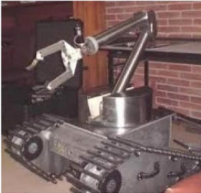
Designed to aid in the cleaning process of landmines in the country without jeopardizing the life of a person, the "**Arcadio**" is a robot developed at the Javeriana University to detect explosive devices underground and off. It is managed by a human being through a laptop from a distance and has intelligent computerized arm.
