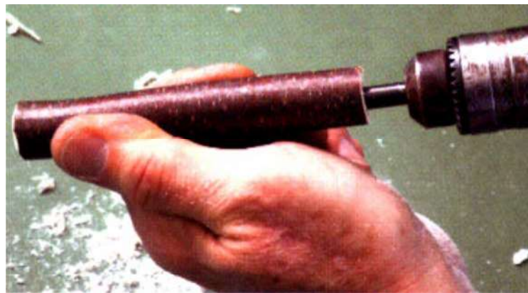
Figure A-2 Drill a Hole
