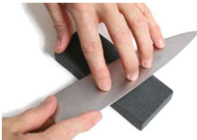
Figure 15 Sharpening the Reverse Side of the Knife
