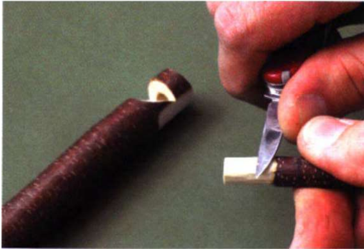
Figure A-7 Whittling a Dowel
