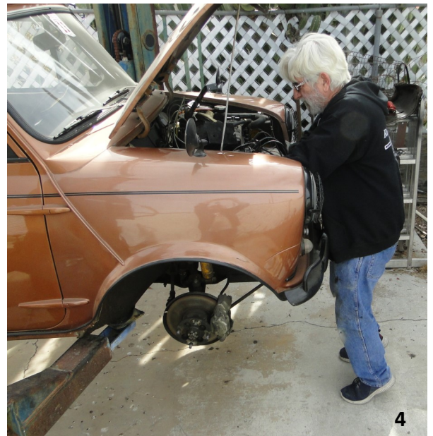
Photos 4 & 5– Changing over from a single brake system to a split system wasn't as straight forward as we hoped (Metric fittings and SAE don't go together).
