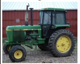
**JOHN DEERE 4440 & 4230 TRACTORS:** 1982 JD 4440, Power shift, 1100 hrs on overhaul w/ 50 series cab, Titan 18.4-38; 1975 JD 4230, Syncro shift trans, open station, Firestone 18.4-34; Buhler Allied 595 quick attach loader w/7' bucket; 12 JD front weights; 4 rear wheel weights; 18.4-38 clamp on duals
