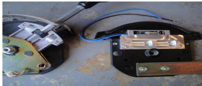
Install the Large billet switch bracket with preinstalled switch with roller facing toward the shifter. Use the 2 supplied  $\frac{1}{4}$ "-20 x  $\frac{3}{4}$ " bolts and star washers thru the existing holes from the outside of the shifter housing.
