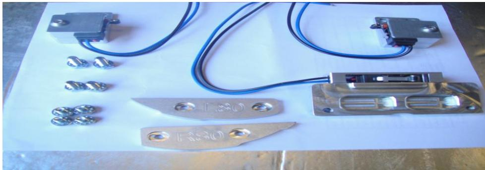
Remove shifter from vehicle. Now remove center bolt from Right side of shifter housing along with Allen head screw at front and rear of shifter. Remove Right side of shifter housing taking care not to lose the star lock washers. (some housings will pull right off some will take GENTLE prying to remove).
